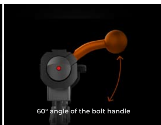
Striker status indicator for a visual and tactile check of the striker mechanism
